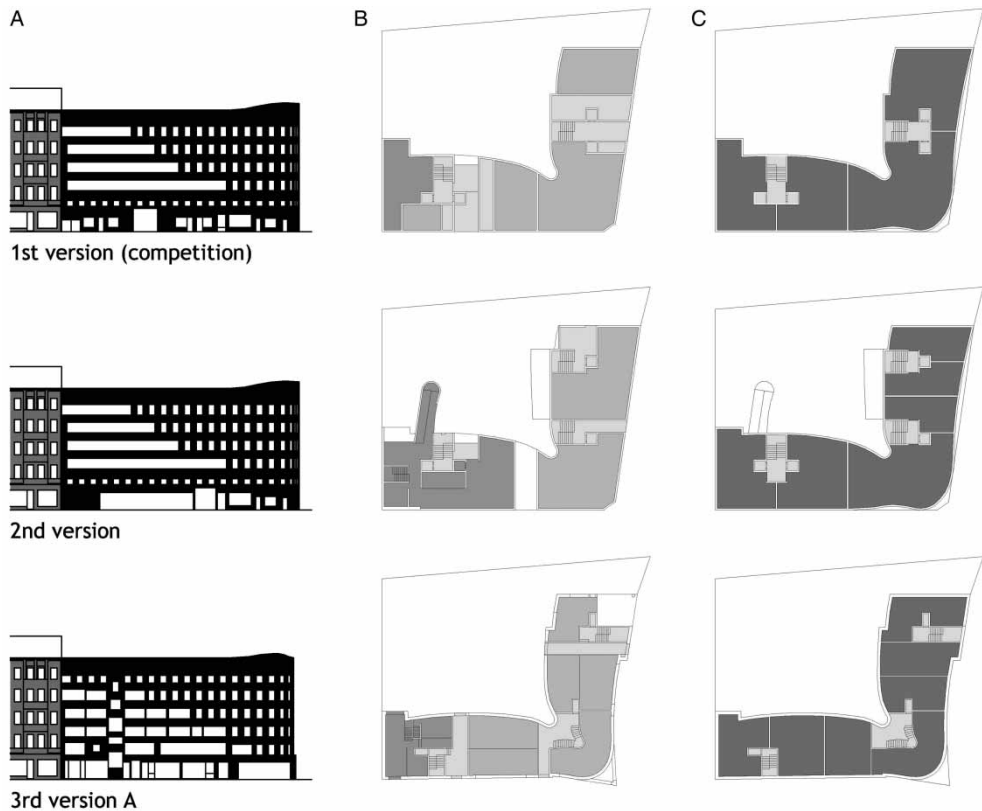
Figure 9. Álvaro Siza, housing block in Schlesiisches Straße, 1980–84: A. elevation Falckenstein Straße; B. ground floor plan; C. typical floor plan (source, Author's drawing).
